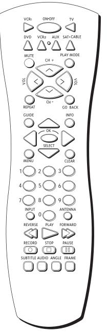
The component buttons are at the top of the remote control, near the ON•OFF button. They are: VCR1, TV, DVD, VCR2, AUX, SAT•CABLE.
